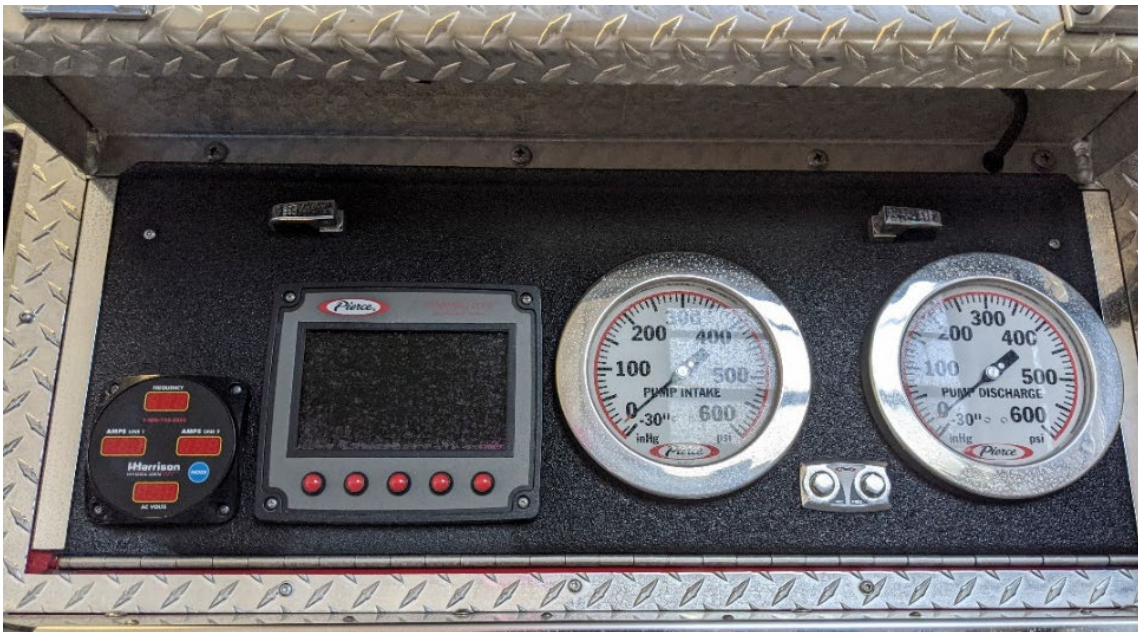
Water spots making the gauges and computer screen difficult to see.
