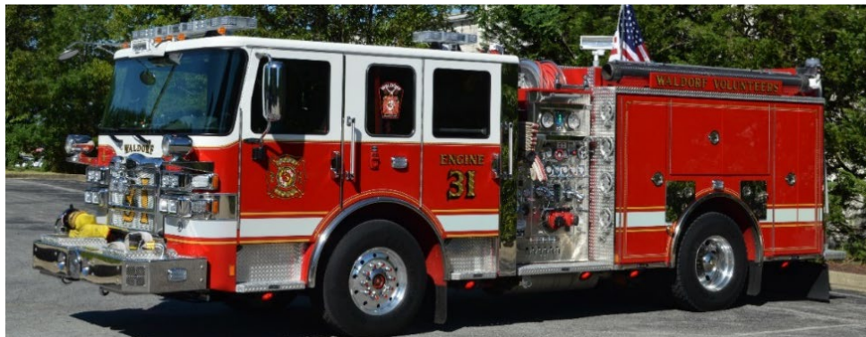
Example of short wheelbase engine with 500-gallon water tank
