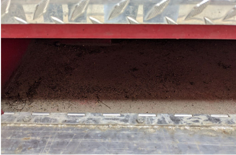
Clean all compartments of dirt and debris
