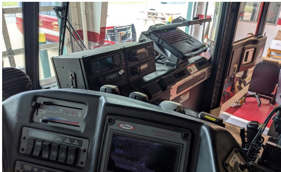
The MDC and mounted radio equipment block the drivers view while driving.
