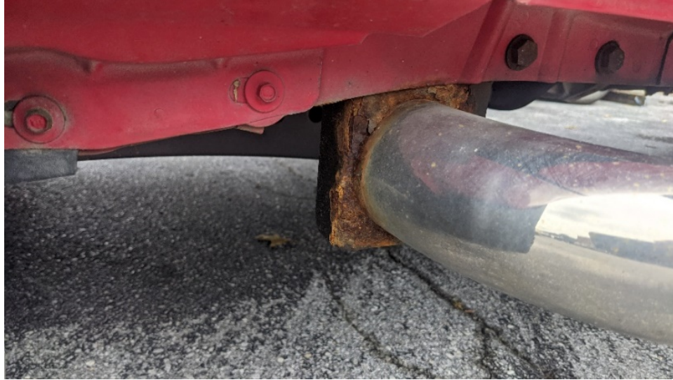
Rust remediation needed on Utility 25 pictured drivers step bracket.
