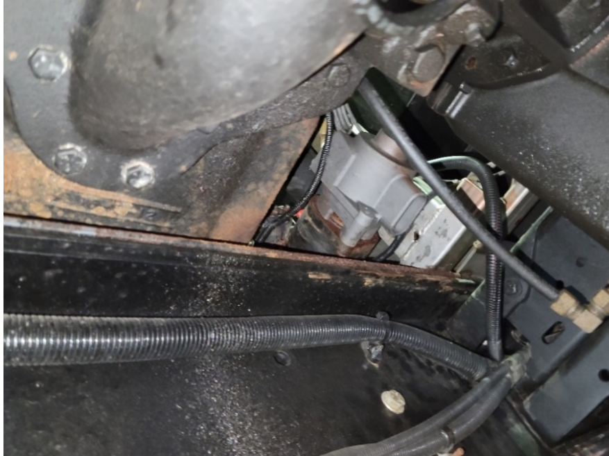
Remediate minor rust on the underside of the apparatus.
