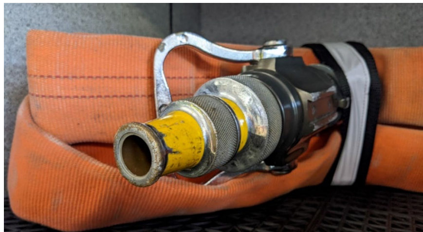
The standpipe pack has a “overhaul tip” on the nozzle.
