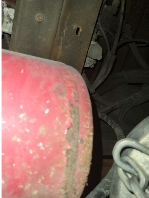
Air holding tank corrosion
