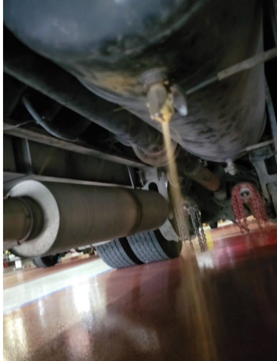
Excessive moisture out of the air brake system holding tank.
