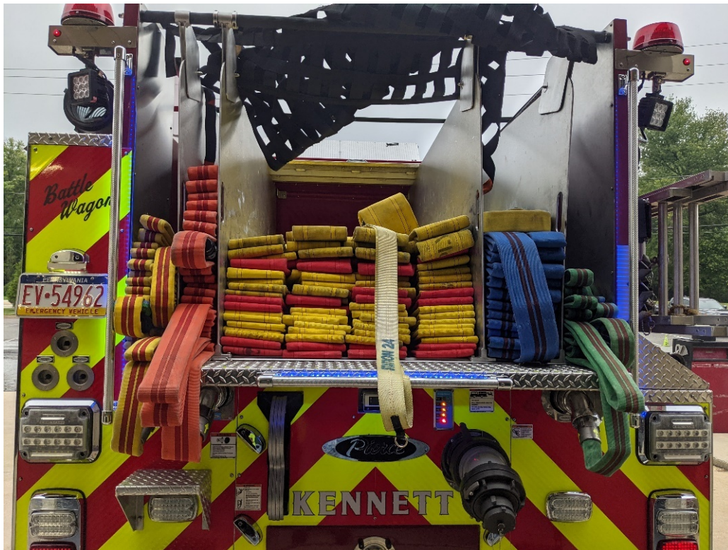
Rear hose bed arrangement on Engine 24
