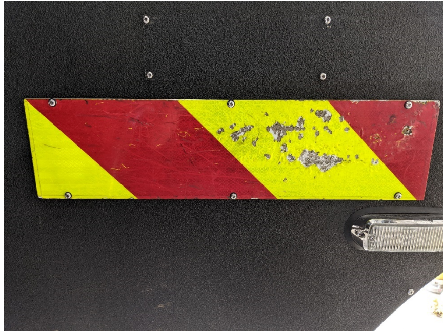
Replace the reflective stripe on the officer's cab door
