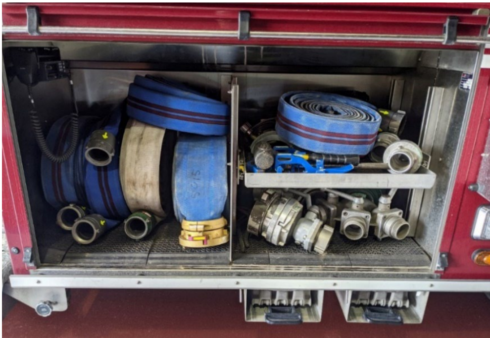
Mount all loose equipment in NFPA approved 9-G Brackets
