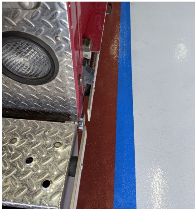
Space rub rails away from the body to protect the rollup door hardware and lift bar latch
