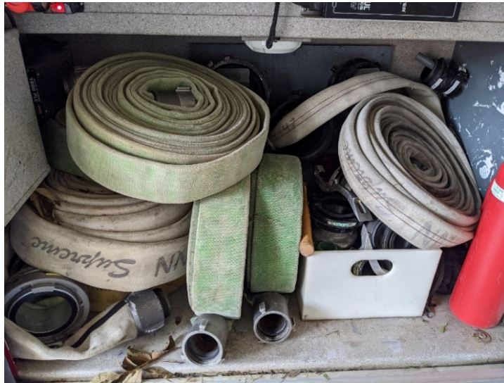
Equipment and spare hose should be secured inside the body compartment
