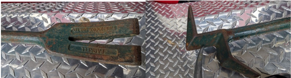
Tools on the front bumper need to be cleaned of rust and repainted.
