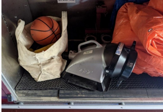
Mount all loose equipment in NFPA approved 9-G Bracket.
