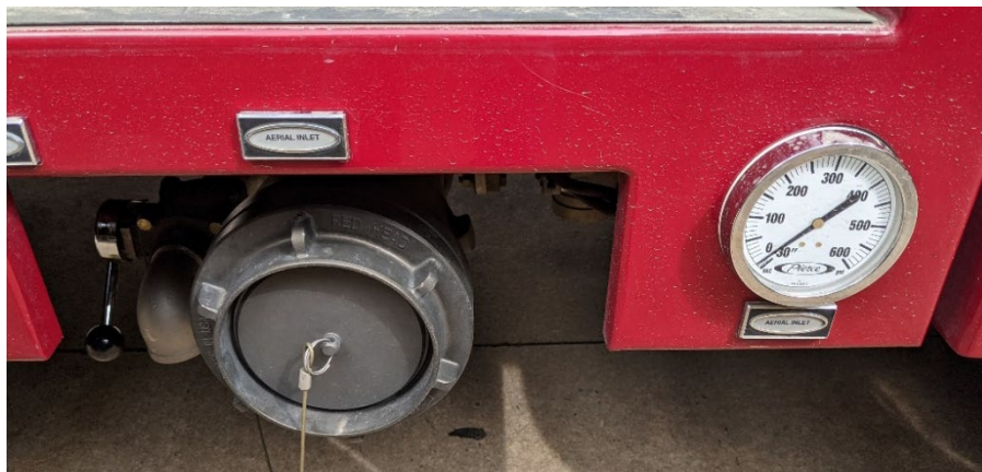
Change aerial inlet gauge to 0-300 psi range
