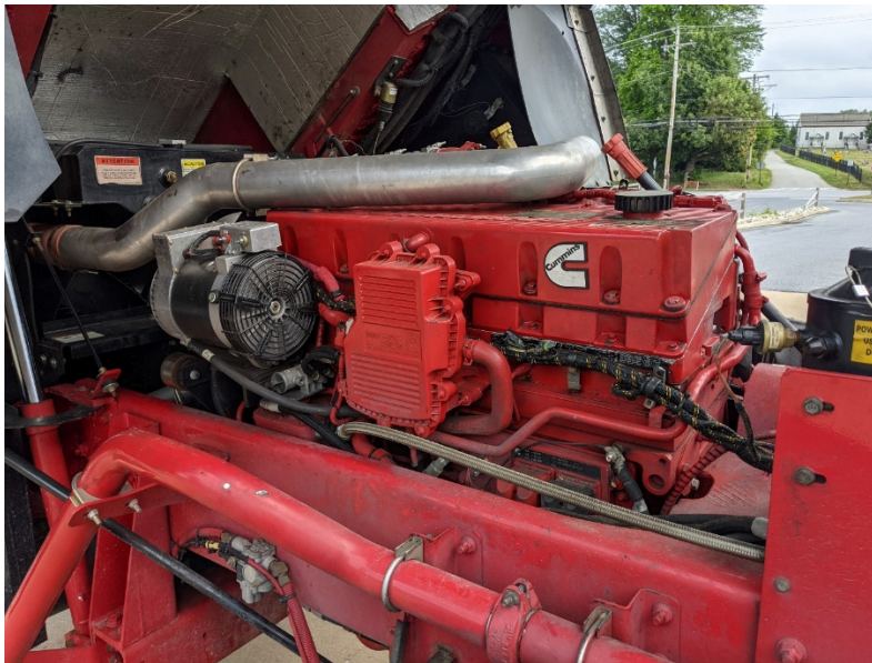
The engine compartment and frame rails show dirt buildup and needs to be steam cleaned.
