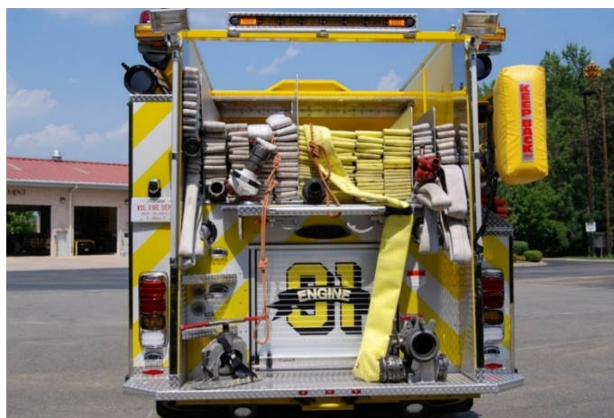
Example of low rear hose bed with 750-gallon water tank
