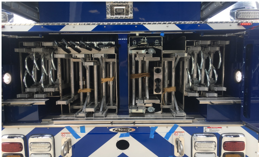
This tractor drawn aerial is equipped with 463' of ground ladders
