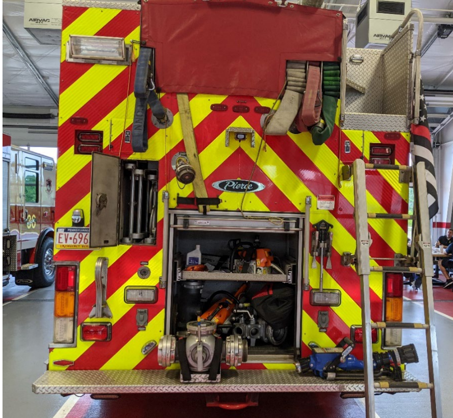
The hose bed is too high off the ground and the hose bed cover prevents rapid, safe deployment of attack lines.
