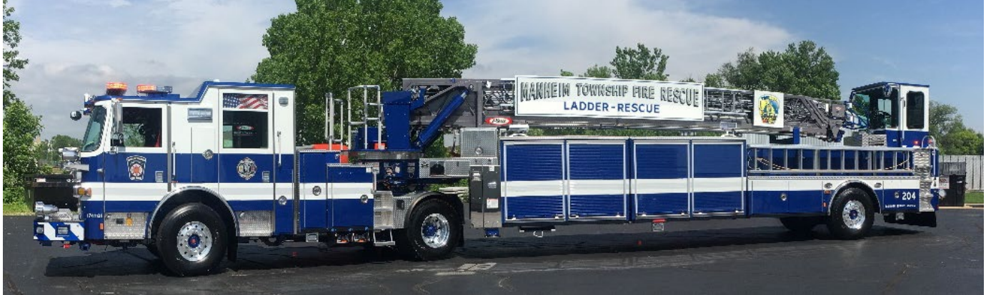
Example of a Tractor Drawn Aerial Ladder that would fit the needs of the Longwood Fire Company. The overall length is 61'3" and the overall height is 136" which would fit in the current fire station.
