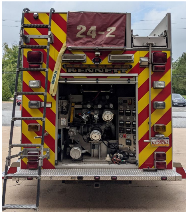
Hose bed too high off the ground making this unit unsafe to work on.
